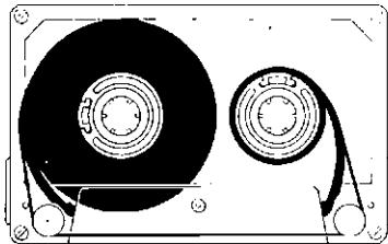
In all new cassettes the neatly reeled tape fits comfortably between the top and bottom of the cassette case. The hubs turn freely. But, after it's unreeled and reeled up again a few times the tape may not wind back as neatly. So that the reel of tape gets fatter and doesn't fit comfortably any more. It starts to drag. And the winding up side goes slower than
